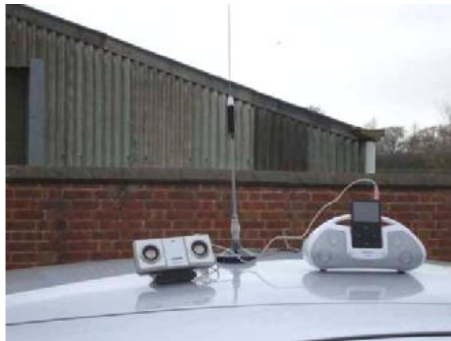
Figure A.3.2.1-24: Creative "Travelsound" (left) and IMOVES "IP300" (right) next to the Transmit antenna
