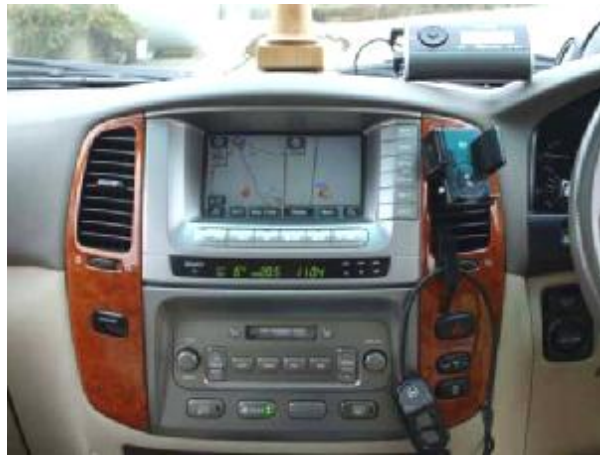
Figure A.3.2.1-7: Standard-fit MW/LW (AM) and Band II (FM) receiver in a Toyota Amazon The Pure Highway DAB receiver is also visible to the top right of the image
