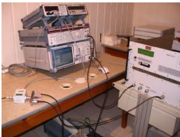
Differential Mode (with Generator SMH)
