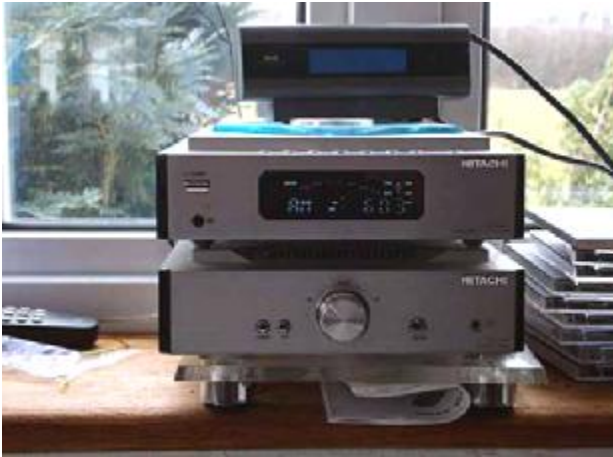
Figures A.3.2.1-16 and A.3.2.1-17: The Hitachi AX-M66 MW/LW (AM) and Band II (FM) receiver and amplifier, with separate Matsui DA-1 DAB receiver on top In figure 17, note the antenna
